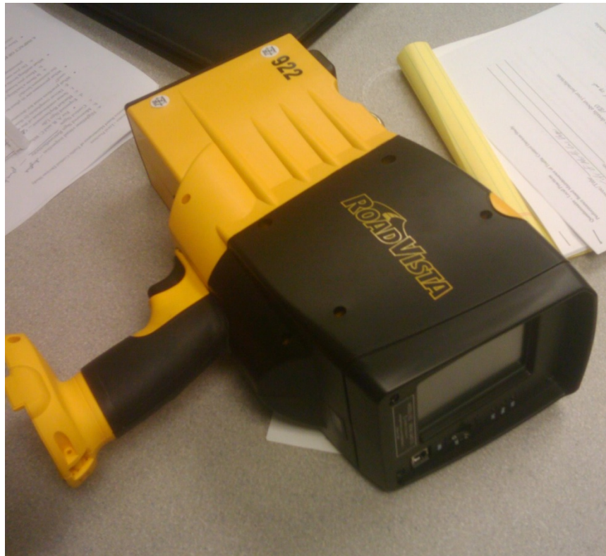
Figure 3: North Las Vegas' Retroreflectometer
